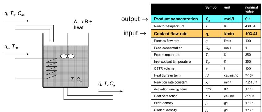
Energy balance equation  $\mathcal{P}(t) = \frac{q(t)}{V} (T_0 - T(t)) + \frac{\Delta H}{\rho C_p} k_0 C_a(t) \exp\left(-\frac{E/R}{T(t)}\right) + \frac{\rho_c C_{pc}}{\rho C_p V} q_c(t) \left[1 - \exp\left(\frac{-hA}{\rho_c C_{pc} q_c(t)}\right)\right] (T_{c0} - T(t))$
