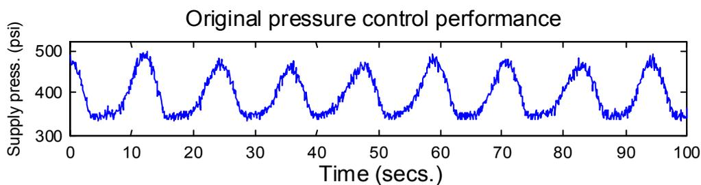
When consulted, the original equipment suppliers had suggested solutions involving significant capital expenditure. However, by building and validating a model of the process with its controls, ISC engineers were able to diagnose the cause of the variations and test a solution without plant intervention. Once developed, the solution, which involved no capital expenditure, was implemented on the plant. Its effectiveness can be reviewed in the trend plot below:
