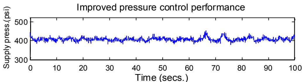
The 80% reduction in pressure variability resulted in significantly reduced maintenance intervention and a substantial saving in the cost of machinery spares.
